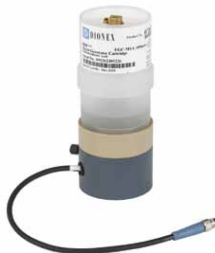
Figure 1. Eluent generator cartridge.
