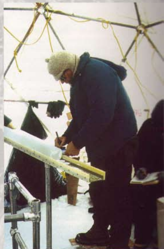
Lonnie Thompson examines stratigraphy of freshly drilled ice core in drilling dome at field site, Dasuopu Ice Cap, Himalayas.
