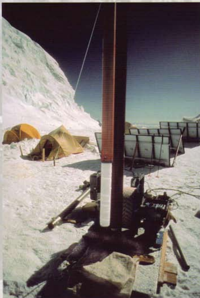
Solar-powered ice core drilling on Nevado Huascarán, Peru. This is the highest tropical mountain in the world.
