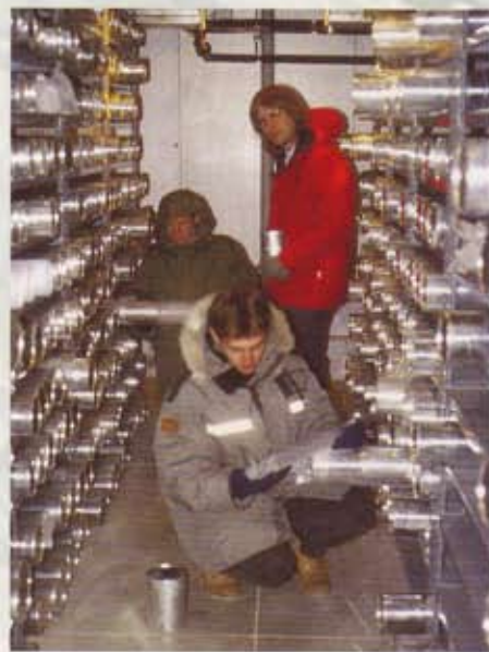
Deep freeze core storage facility (-30 to -40 °C) at Byrd Polar Research Center, Ohio State University.
