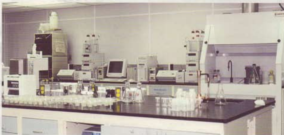
Class 100 clean room with Dionex DX-500 ion chromatographs at Byrd Polar Research Center, Ohio State University.
