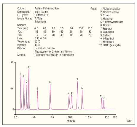
Figure 2. Carbamate pesticides listed in EPA Method 531.2, separated using a  $3.0 \times 150$  mm Acclaim Carbamate column.
