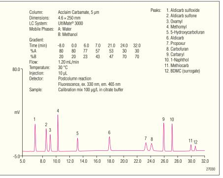
Figure 1. Carbamate pesticides listed in EPA Method 531.2, separated using a  $4.6 \times 250$  mm Acclaim Carbamate column.
