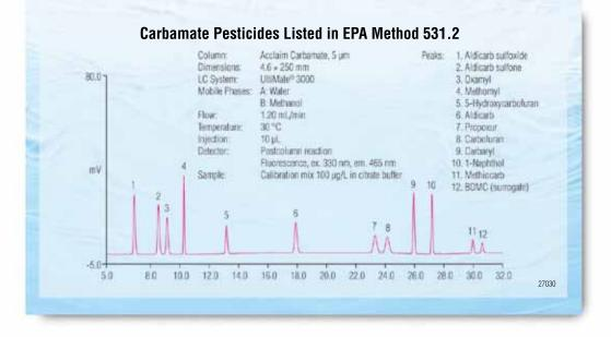
The Acclaim<sup>®</sup> Carbamate columns are designed for the baseline separation of carbamates specified in the U.S. EPA Method 531.2, using LCpostcolumn derivatization-fluorescence or LC-MS detection.
