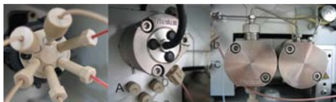
Figure 1. The UltiMate 3000 Titanium system features titanium pumps and PEEK fluidic path.
