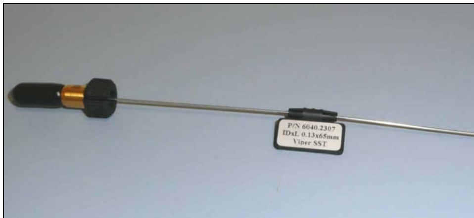
Figure 8: Removable labeling clip with sticker for individual capillary labeling.
