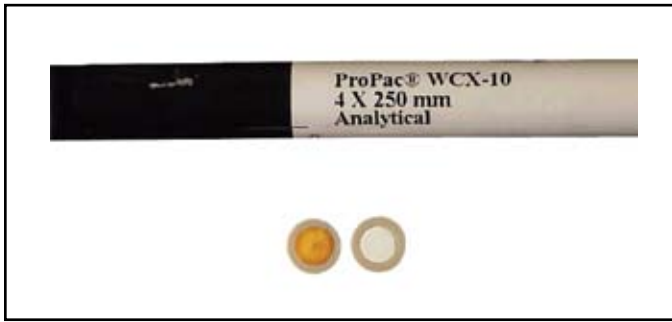
Figure 7. A picture of inlet frit of ProPac WCX column after Fe^{3+} loading experiment (left). An unused frit is shown for comparison (right).
