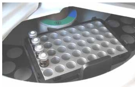
Fig. 22: Inserting a vial tray
