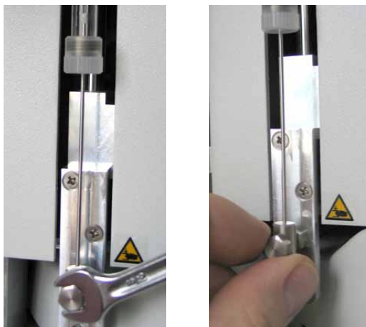
Fig. 40: Disconnecting the syringe on the plunger
