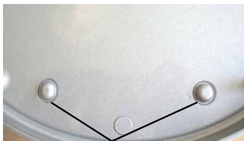
Locking pins on the carousel bottom
