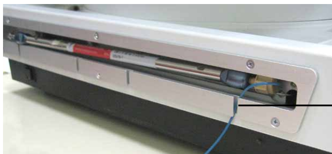
Fig. 14: Column in column chamber
