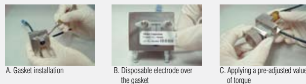
Figure 3. Installation of Disposable Electrode in Amperometric Cell
