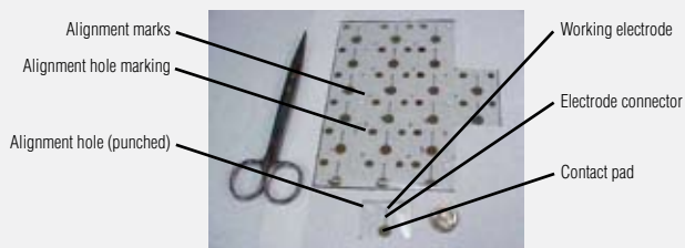
Figure 2. Disposable Working Electrodes* on a Polymeric Substrate
