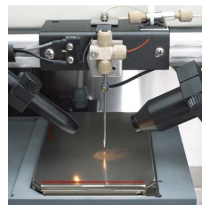
Fraction collection on a Bruker AnchorChip MALDI target. The Probot is equipped with an optional video camera for viewing the spotting remotely.
