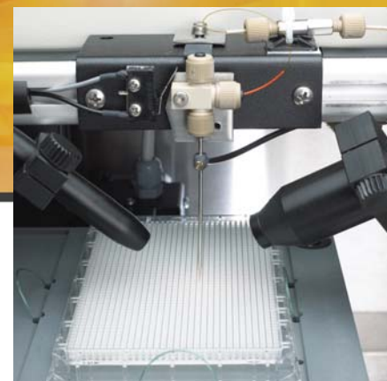
For multidimensional LC applications, the Probot can be used to collect fractions into microtiter plates.
