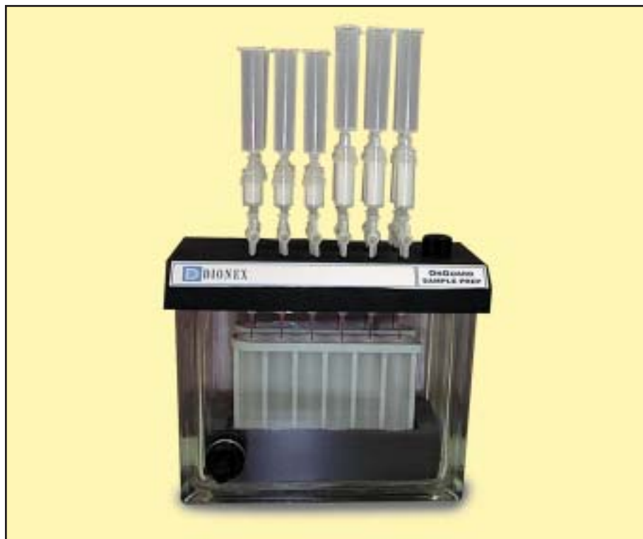
Figure 7. Samples can be processed in parallel using the OnGuard Sample Prep Station.
