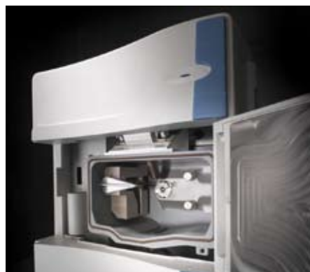
MSQ Plus source design features tool-free maintenance.
