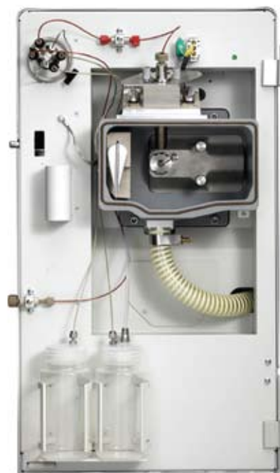
Reference inlet system — calibrant bottles (lower left), flow switching valve (upper left), and source inlet (center).
