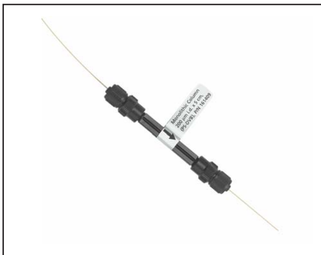
Figure 1. Monolithic column in protective housing.
