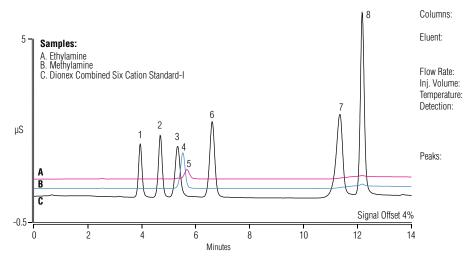
Figure 3. Separation of six cations, methylamine, and ethylamine on the Dionex IonPac CS12A column.
