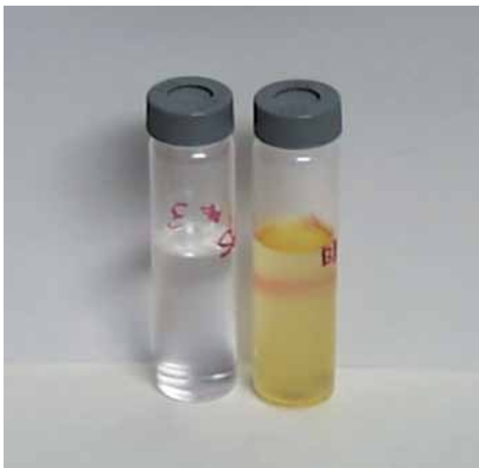
Figure 5. Extracts with and without in-cell cleanup of fish tissue using alumina, silica gel, and acidic silica gel (40% H_2SO_4 ).
