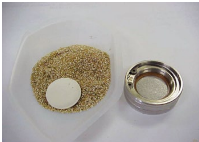
Figure 2. Due to the complete neutralization and absorption of the acidic sample by the resin method, no coloration is observed on the frit or on the filter.
